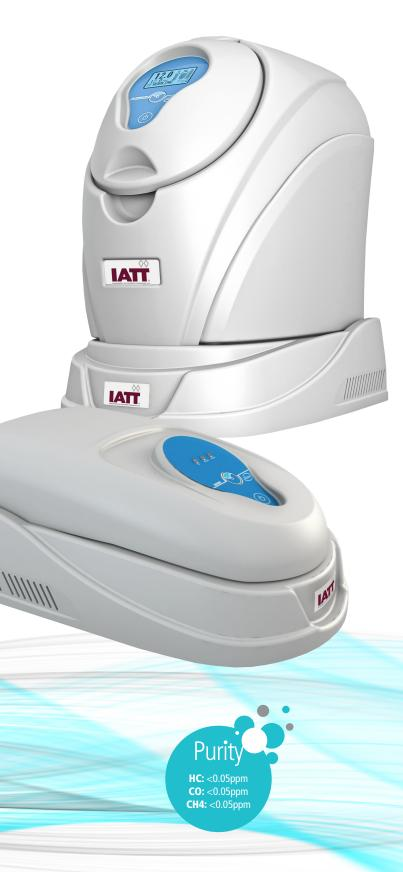
AiroGen® Zero Air Generators from IATT produce dry and hydrocarbon-free (HC) air < 0.05 ppm, using a heated catalytic technology from a supply of clean, dry compressed air. The generator can be used individually or coupled to any one of the Modular Hydrogen Generators to form an all-in-one FID gas station solution.
